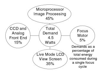
Figure 4: Power consumption breakup inside the Nikon Coolpix camera
