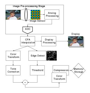
Figure 1: Image processing pipeline in a digital camera
