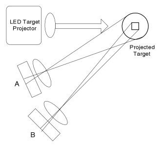
Figure 3: Visible ranging AF system in the DC 260. 'A' is a linear pixilated sensor, which measures the diameter of the projected target; 'B' is a similar detector, which measures the diameter of the inner projected image. In the DC260, the two sensors are part
