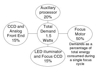
Figure 5: Power consumption breakup inside the Kodak DC-260 camera
