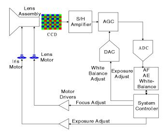
Figure 2: Expanded view of the image pre-processing stage
